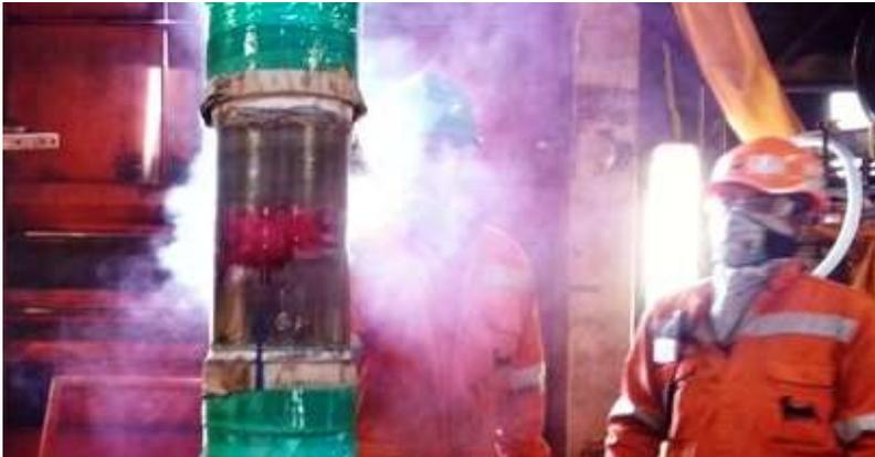
*Cracks on pipe shown at +120°C (+248°F) with dual-response fluorescent magnetic powder Elite FW1AC concentrate for water dilution*
